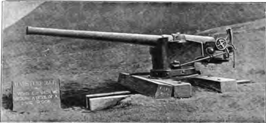
A 4.7 GUN ON TEMPORARY PLATFORM
